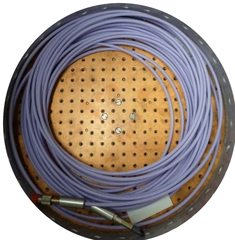
Figures 11 a & b: a) CarlisleIT LITEflightND cable terminated with FC and AVIM connectors by GSFC, b) optical fiber TVAC feedthrus as fabricated and designed for ATLAS by NASA GSFC
