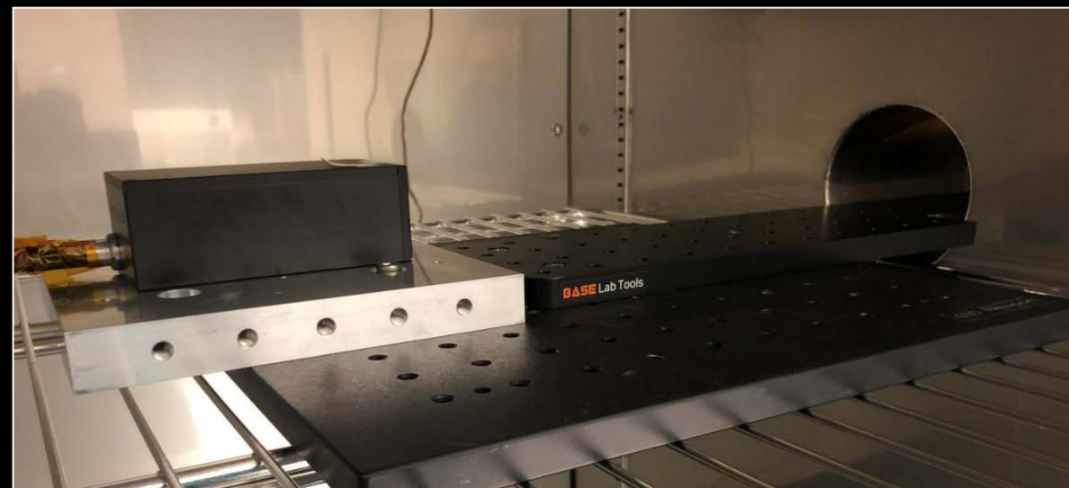
Mini LiDAR in thermal chamber pointed to a target at then end of the chamber feedthrough hole.
