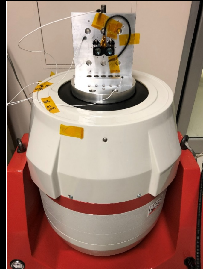
Garmin candidate 2 on vibration shaker
