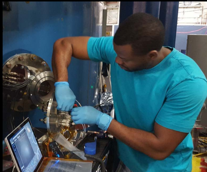
Eleanya Onuma installs vacuum feedthroughs
