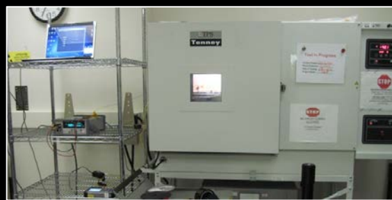
White Light LED Testing in Environmental Chamber
